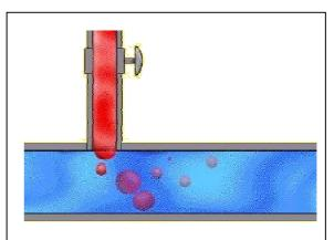
Normally flash will form bubbles and collapse. Sparging is needed to stop hammering.
