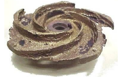
Fig 9 Worn impeller from condensate pump
